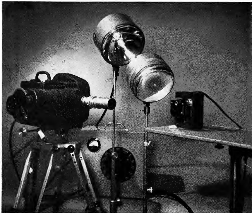
Fig. 1. Setup using the PAR 64 bulb and a condenser. The voltage to the bulb is controlled by a 20-amp variac as shown.
